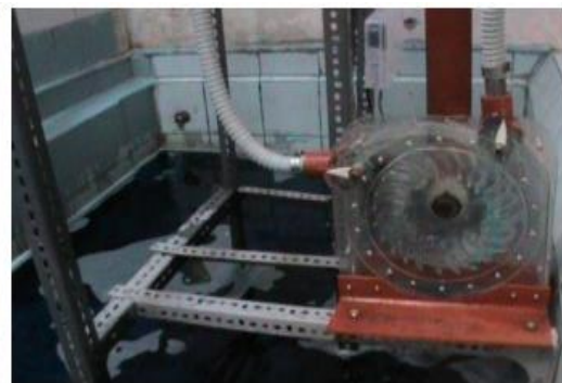
(b).Dual Nozzle Cross Flow Turbine Installation
