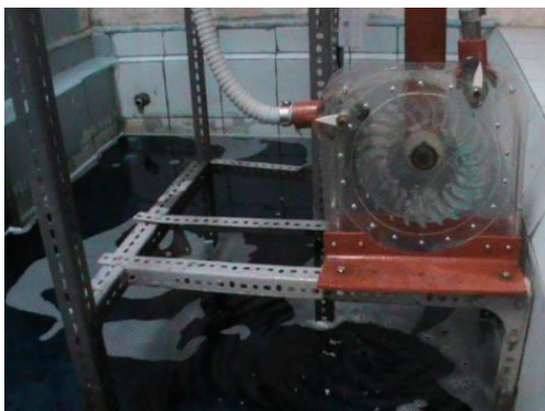
Figure 4. Experiment set-up: 1. Double nozzle/jet cross-flow turbine [6]
