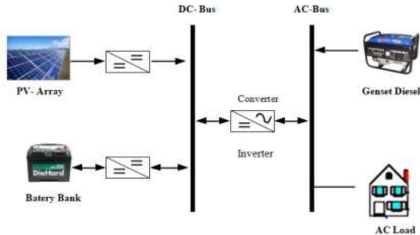
**Figure 3.** Centralized AC and DC coupled hybrid generating systems (Centralized AC and DC-coupled Hybrid Power Systems)
