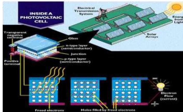
**Figure 1.** Working principle of photovoltaic cells.
