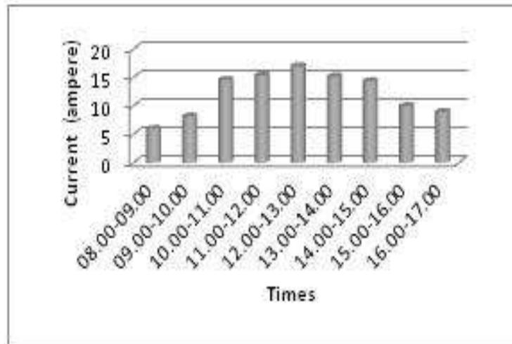
**Figure 7.** The current of the PLTS Hybrid system with Genset
