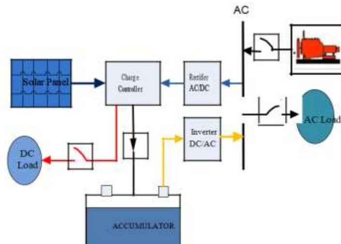
**Figure 4.** Hybrid system scheme for PLTS and PLTD/Genset
