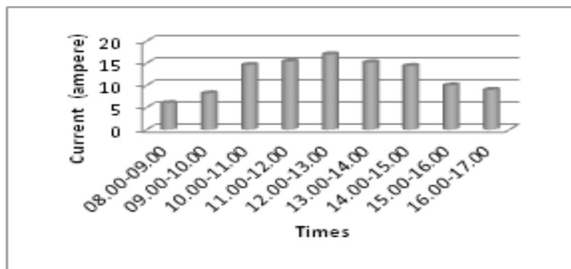
**Figure 7** The current of the PLTS Hybrid system with Genset
