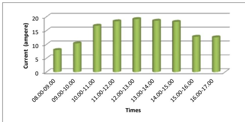
**Figure 6** The current of the Hybrid PLTS system with Genset
