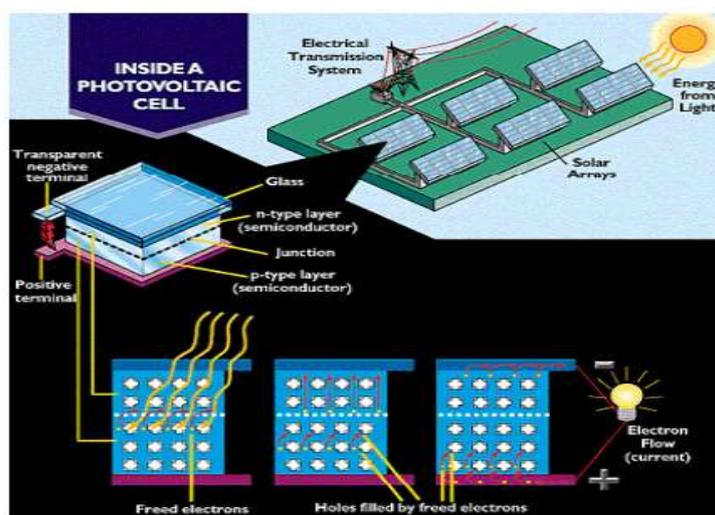
Figure 1 Working principle of photovoltaic cells. [8]
