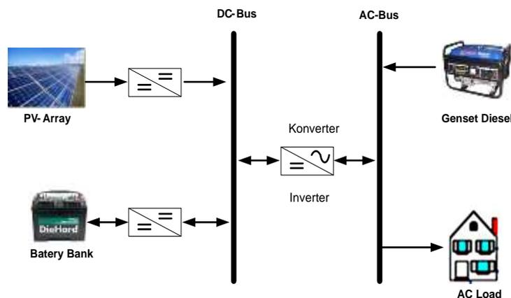
Figure 3 Centralized AC and DC coupled hybrid generating systems (Centralized AC and DC-coupled Hybrid Power Systems)
