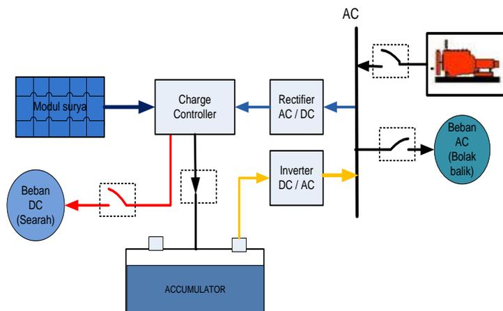
**Figure 4** Hybrid system scheme for PLTS and PLTD/Genset
